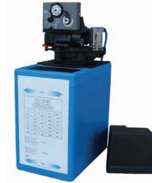
Water softener with automatic regeneration of resins through sodium chlorite for consumption above 800 liters
