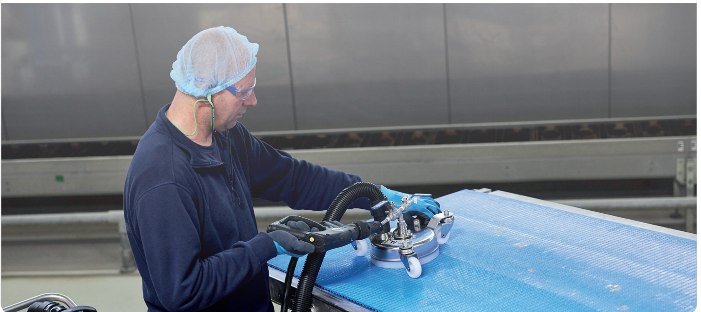
Example of surface cleaner with Radames adapter
